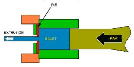
Figure 1: Direct extrusion process
