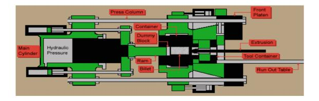
**Main Cylinder**- Chamber and cylinder of an extrusion press into which hydraulic fluid is pumped to generate the desired ram pressure and movement.
