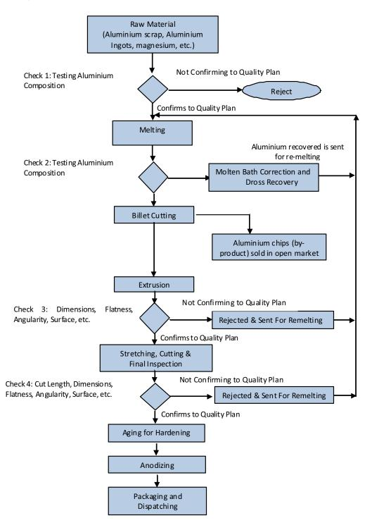
The steps in the manufacturing process are as under:
