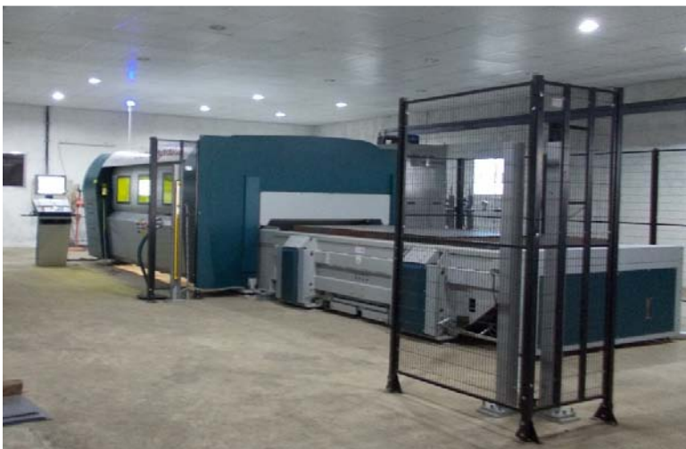
Salvagnini L3 Optical Fiber Laser Cutting Machine Bought From Salvagnini Italia Spa, Italy.
