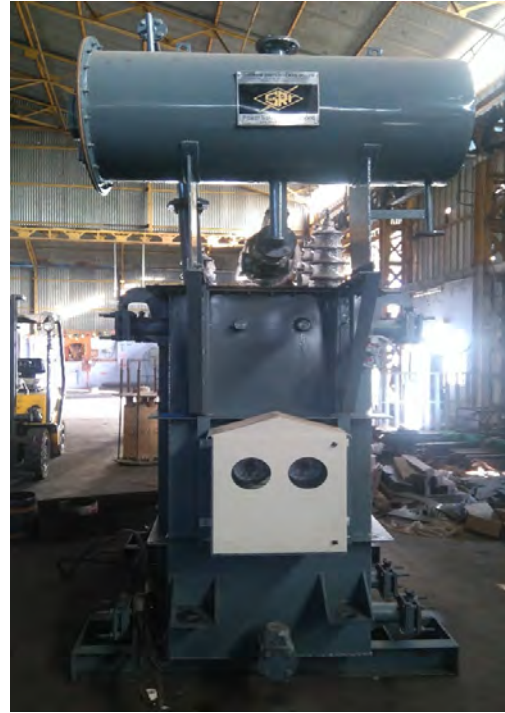
EHV Transformer of 5 mVA Capacity
