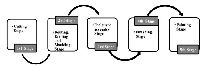
• Cutting Stage – This is the initial stage of loudspeaker manufacturing process. At this stage plywood or MDF Sheet is cut into required shapes and sizes according to different models.
